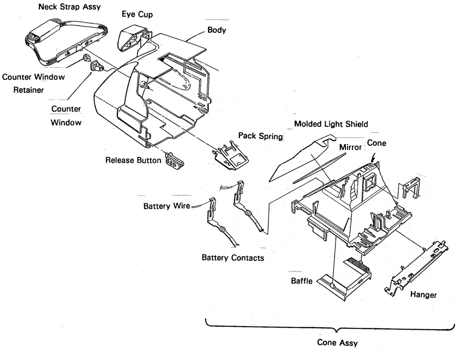
13. To remove the Cone, insert a flat blade screwdriver at the locations shown in Fig. 13, springing out the sides of the Body slightly. This frees the Cone from the catches inside the Body. Lever the Cone forward, out of the Camera Body. The freed Release Button will drop out.
