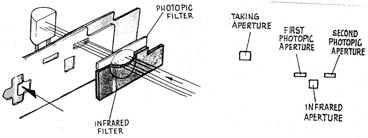
41. For low light FAR pictures, the blades travel even farther. First, there is a very small amount of light passed through the first photopic aperture. Next, a very small amount of light passes through the infrared aperture. Finally, the blades open fully and a large amount of visible light passes through the second photopic aperture. The exposure shutdown is dependent on the measurement of this combination of light (or on clock time-out).
