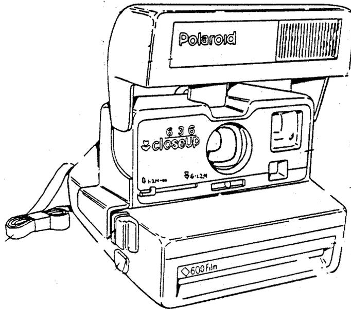
7. When you open the camera, you can see another obvious difference between the Model 636 and the One Step — a built-in electronic flash. The flash is designed to be used for all pictures, both indoors and outdoors.
