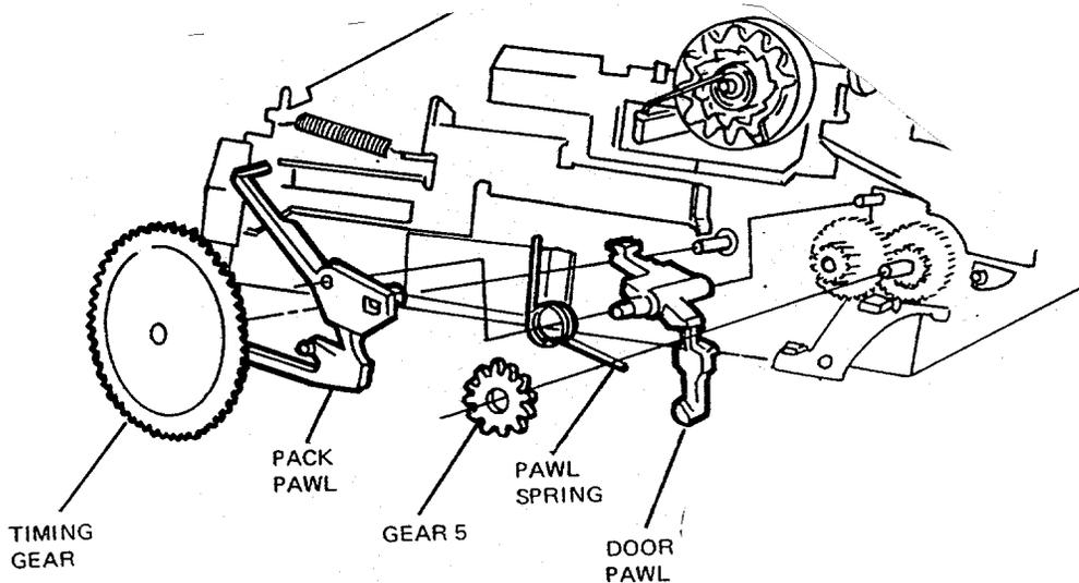
Fig. 42 Parts removal from Gear Drive
