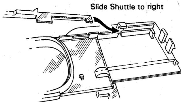
Fig. 12 Replacing the Shuttle in the Close Up Lens
