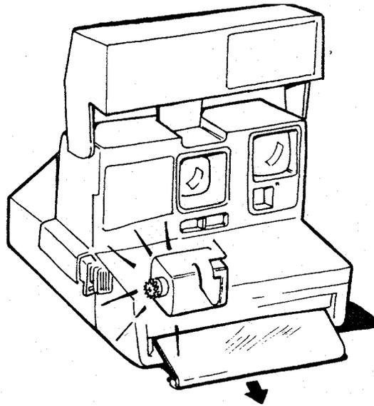
8. After the blades close, the motor is turned on, activating a gear drive system similar to the system in the OneStep. The timing gear:
