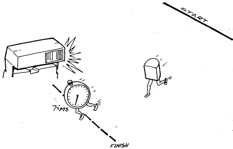
23. The next condition in which a flash exposure can be made is in a low ambient condition (low light level, outdoor scenes and all indoor scenes). In this condition, there is so little light that the clock beats the photocell in the race to fire the flash. When the clock reaches 74 milliseconds (ms), the flash is fired.
