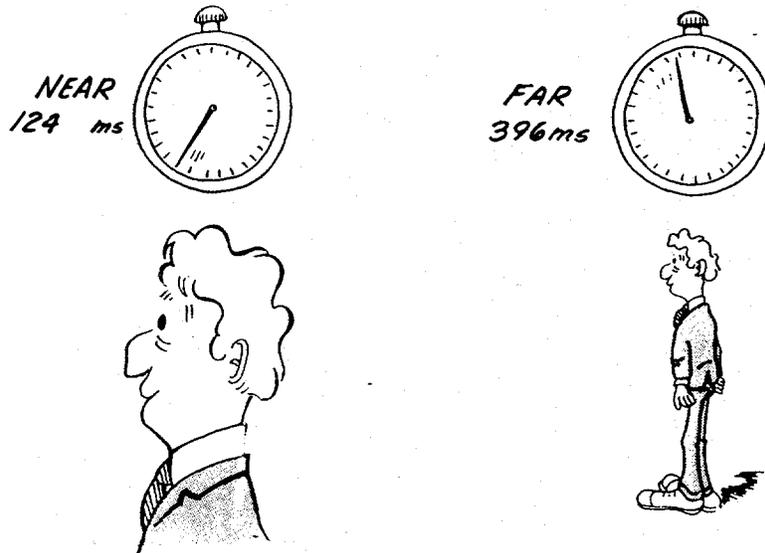
27. For NEAR subjects the logic instructs the clock to stop the exposure at 124 ms after the blades open. For FAR subjects the clock will time-out at 396 ms to stop the exposure.
