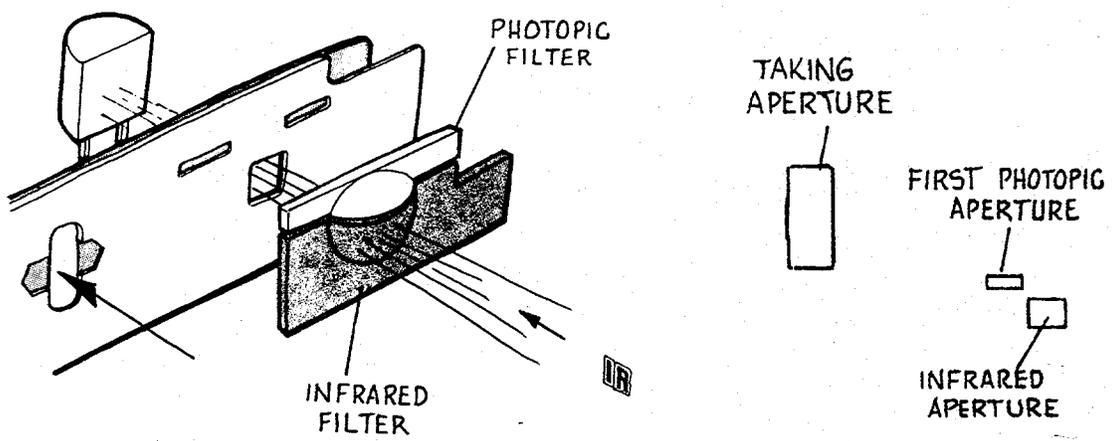
40. In a low light NEAR shot, the blades travel farther. During blade travel a very small amount of visible light passes through the first photopic aperture. The blades move to the position shown, the strobe fires and a larger amount of infrared light passes through the infrared aperture to the photocell. Exposure shutdown is dependent upon the combination of an extremely limited amount of visible light added to the larger amount of infrared light (or on the clock time-out).
