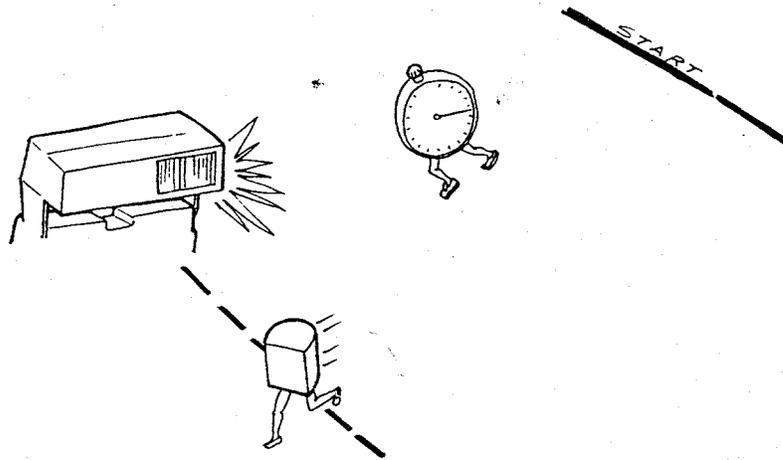
19. Now, let's go back to the three conditions in which a flash picture can be taken. The first is in high ambient light. In this condition, there is so much scene light available that the photocell always wins the race to fire the flash. This is the Fill Flash mode of operation.
