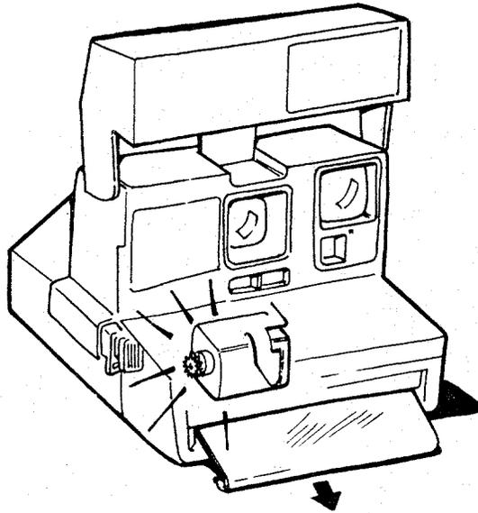
13. After the blades close, the motor is turned on. The timing gear advances the pick, indexes the counter, and brings the S5 actuator back to its original position. The shutter system is latched closed, ending the low ambient NEAR sequence.
