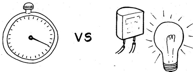
28. However, the ending of the exposure is also subject to the photocell light measurement. In other words, for a Low Ambient NEAR or FAR picture, there is still a race between the photocell and the clock to shut down the flash and close the blades.
