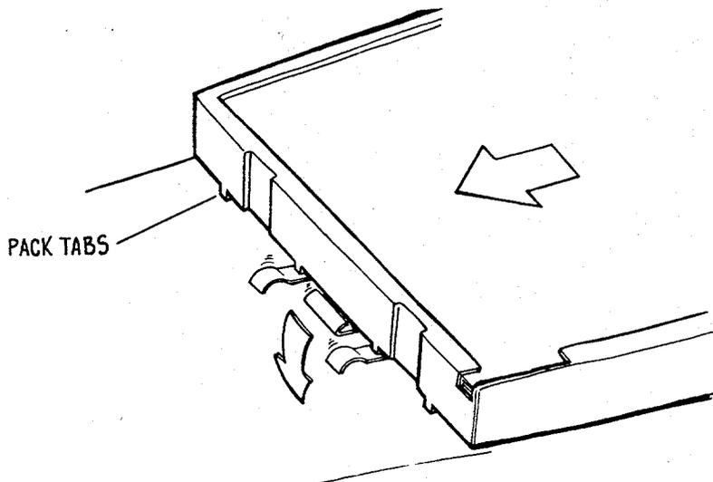
4. On the inner edge of the 600 film pack is a set of molded plastic tabs which interface with the pack spring in the camera. The two middle tabs press down the ramps of the pack spring, allowing the film pack to slide over the stop for insertion into the camera. On older style SX-70 packs there are no tabs. As a result, the pack is prevented from being inserted into a 600 line camera by the pack spring stop.
