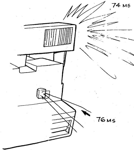
25. The question is answered by measuring the amount of light seen by the photocell two milliseconds after flash fire.
