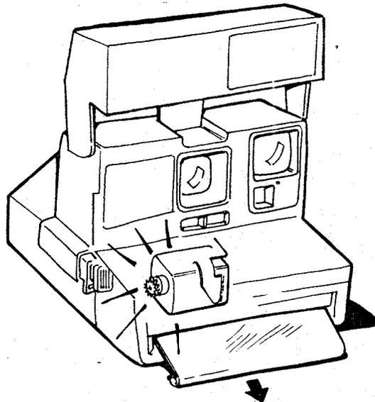
16. After the blades close, the motor is turned on. The timing gear advances the pick, indexes the counter, and brings the S5 actuator back to its original position. The shutter system is latched closed, ending the low-ambient FAR sequence.
