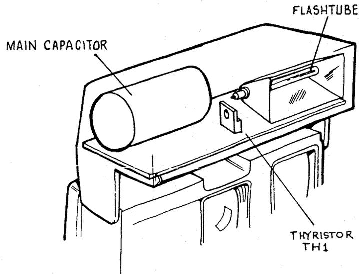
12. Whether or not the flash provides full output, the main capacitor delivers the same amount of energy. Therefore, if the flash is ordered to shut down early, some means must be found to dissipate the remaining energy in the circuit. This remaining energy is diverted through a thyristor (TH1) on the strobe board.
