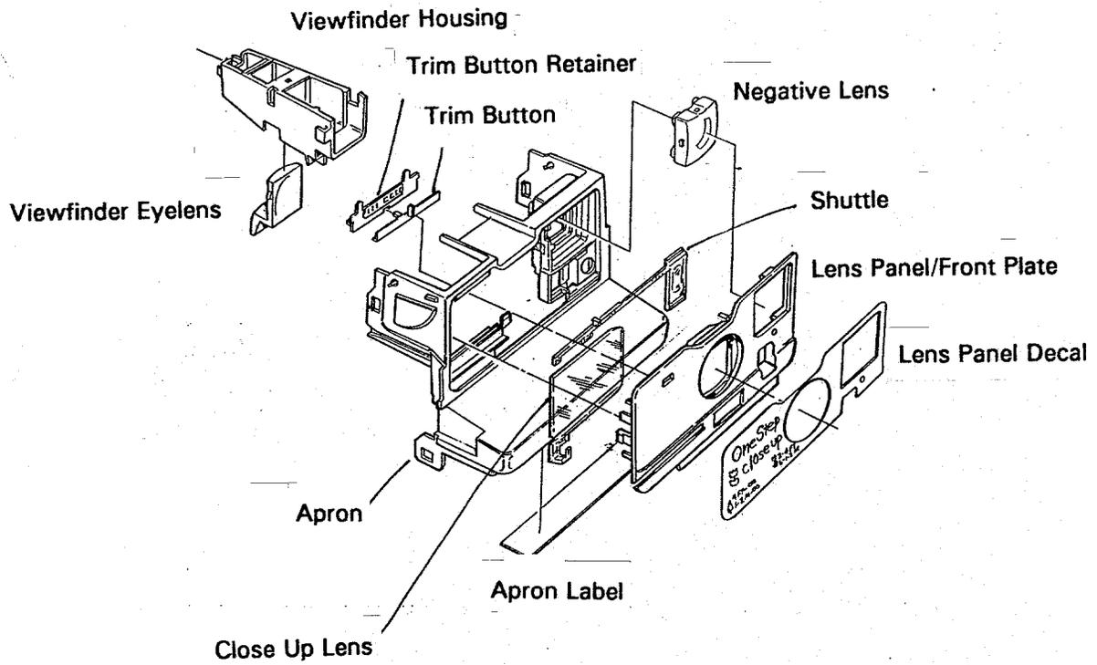
8. Open the Film Door to remove the Apron. Insert a soldering aid, first at position A and then B (Fig. 8), to free the Body detent lugs from the Apron. Carefully “lever” the Apron out of the Body. Repeat the process on the opposite side. The S1 Button and S10 Button with Return Spring will fall out.
