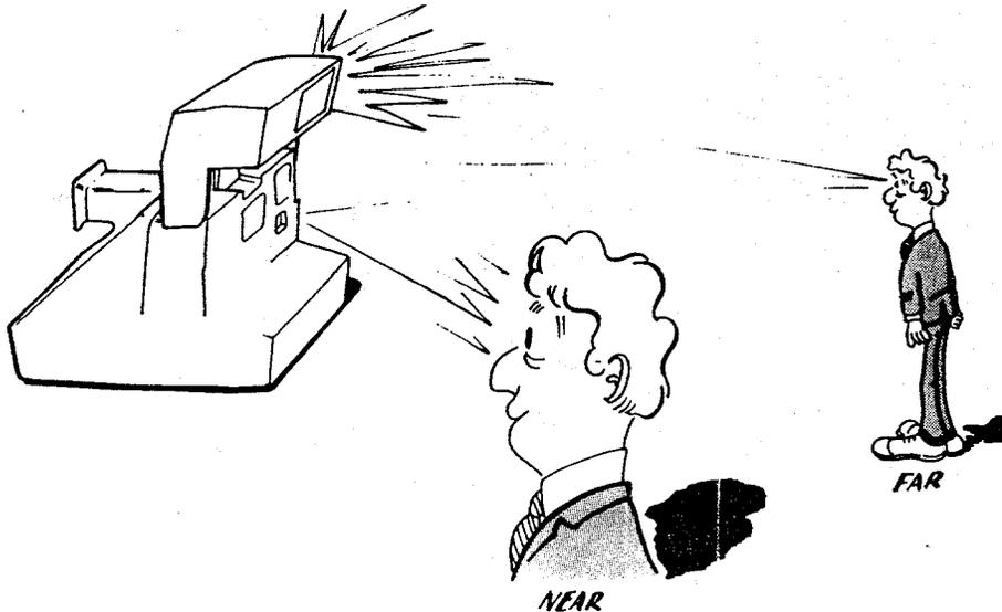
24. Two milliseconds after flash fire, a very important question is asked by the camera logic: Is the subject near or far? The answer is needed to properly set the clock for time-out.
