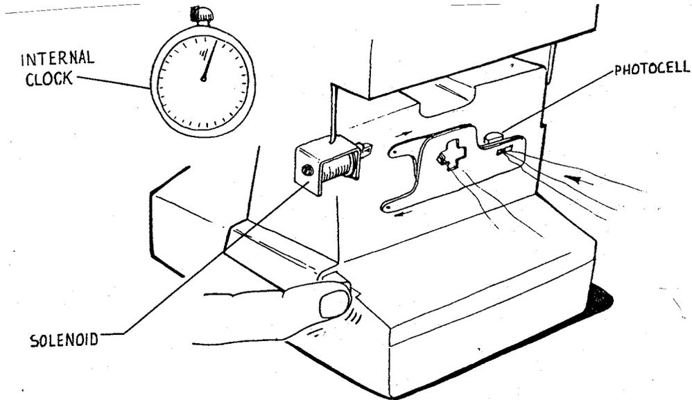
17. After the flash is charged and the exposure button is pressed all the way in, three things happen simultaneously which decide how the flash is going to be controlled:
