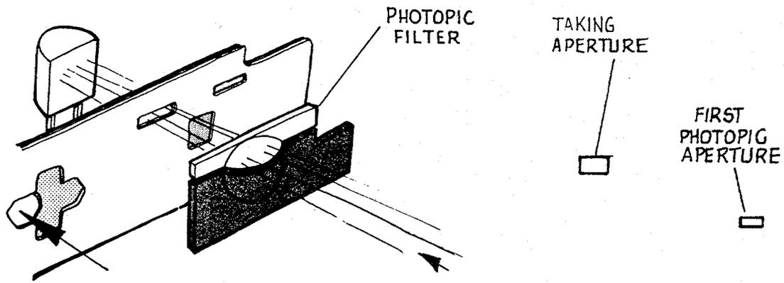
39. For Fill Flash pictures, the shutter blades open as shown here. The blades are set so only visible light passes through the first photopic aperture to the photocell. Thus, for Fill Flash, exposure shutdown is based on the measurement of visible light only.
