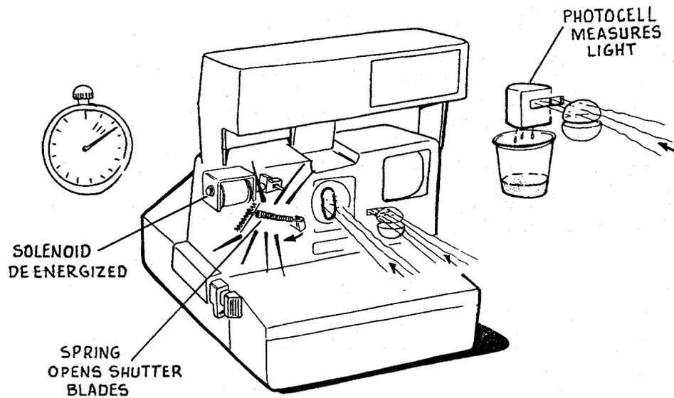
5. With the solenoid deenergized and the walking beam free of the shutter latch, spring-action opens the shutter blades. The internal clock is running and the photocell starts to measure light.
