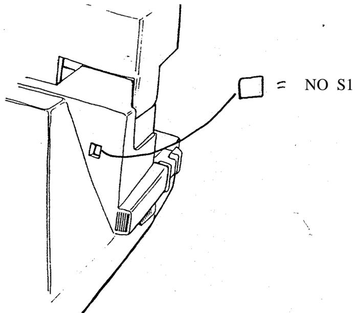
45. There are two mechanical inhibits. When the counter reaches its blank setting, S1 is prevented from closing. This is the same as the empty pack lockout feature on Pronto! cameras.
