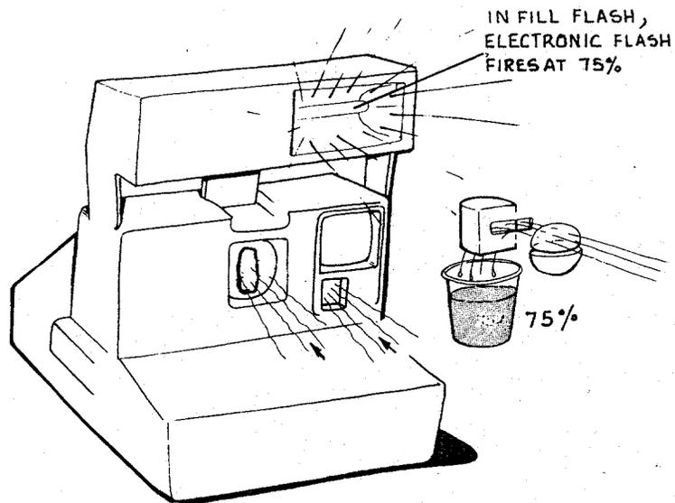
6. In a fill-flash exposure, when the photocell sees 75% of the light needed for a proper exposure, it signals the flash to fire. The flash provides the remaining 25% of the necessary light. Note that in a fill-flash exposure, the photocell always beats the internal clock in ordering flash fire.
