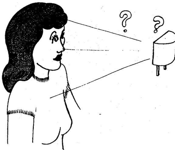
34. This was especially true of flash pictures taken of subjects close to the camera. Light-colored clothing would reflect too much light to the photocell causing it to stop the exposure too soon.
