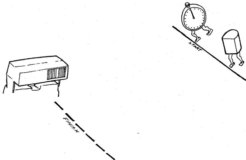
18. From this point, there is a race between the internal clock and the photocell to decide which is going to control the flash. Either the internal clock will time-out before the photocell measures a pre-determined amount of light or vice versa. Whichever occurs first will fire the flash.
