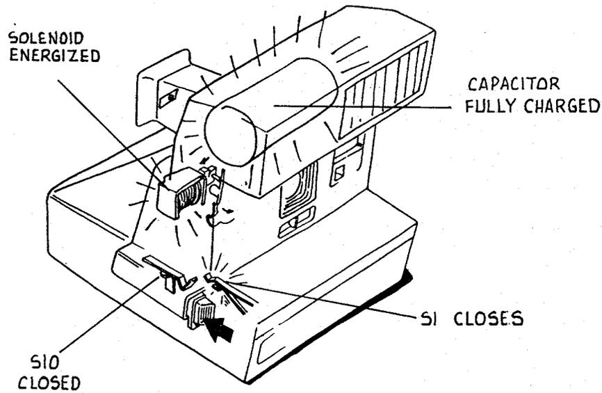
3. Within five seconds the green LED at the rear of the strobe comes on, indicating that the main capacitor is fully charged. The picture taker may now press in the exposure button fully. This closes S1 and S10 remains closed. Closing S1 energizes the solenoid which pulls in slightly.
