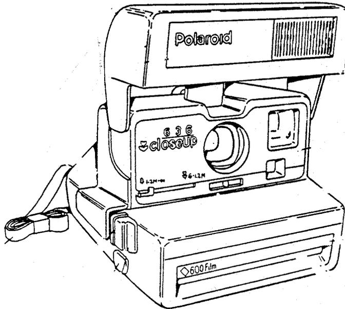
11. The built-in flash is an electronic quench-type flash. It can provide a full output of about 340 zonal-lumen seconds (ZLS) to illuminate a scene or it can be shut down early to provide less light to the scene. The way the camera decides to provide full or partial light output will be discussed later.
