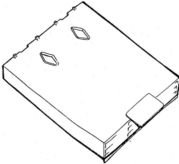
3. One of the major differences between the Model 636 and the OneStep is the type of film it uses. Like all of the 600 line, the 636 uses a new film format. The film has a speed of 600 ASA.
