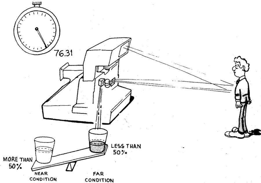
14. If the light measured 2 milliseconds after the flash has fired is less than 50% of the total needed for a proper exposure, the camera decides the subject is FAR.
