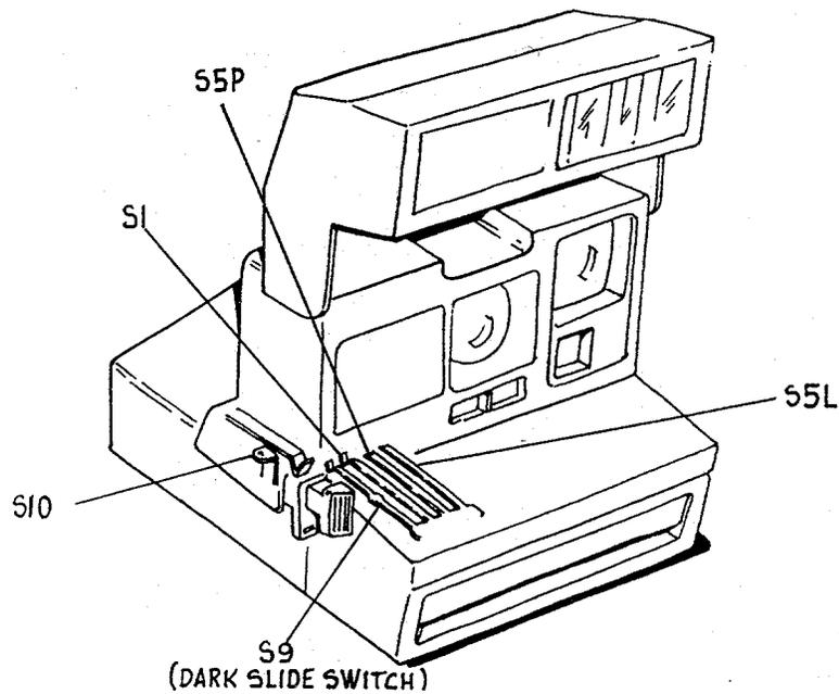
1. Shown here is the location of the switches which regulate flash charging, flash fire and exposure. We will now run through a flash exposure sequence.
