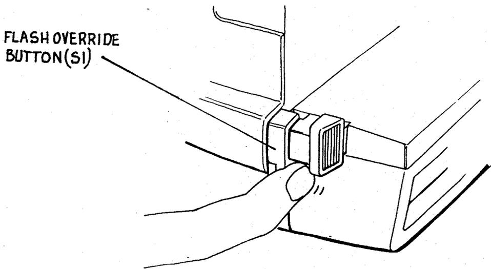
42. The flash may be bypassed on those rare occasions where it is not desired. This is pretty much limited to taking pictures in daylight through a window. In this condition, the flash can be prevented from firing by pressing only the back part of the exposure button. Exposure shutdown is determined by the photocell seeing 100% of the light required for a proper exposure or by the internal clock timing out at 396 ms.
