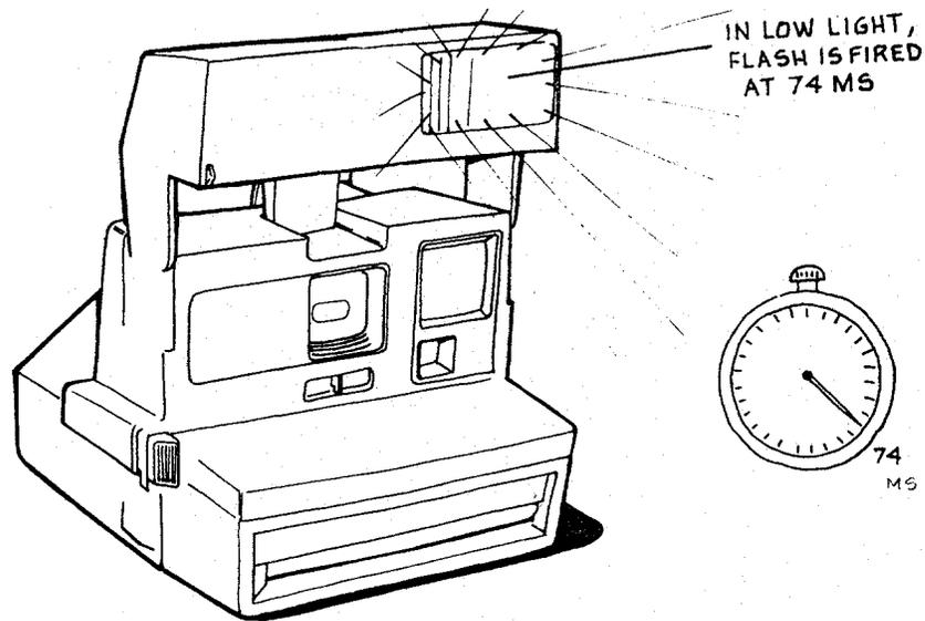
9. The sequence for low-ambient conditions begins identically to the fill-flash sequence. The flash is charged via S10 and the shutter blades open the same way. However, the flash is fired by the internal clock reaching 74 ms, rather than by the photocell light measurement. This happens because there is relatively little light passing through to the photocell.
