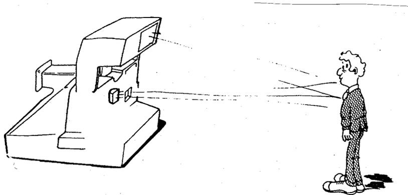
21. At this point, the blades are still open and the exposure is being made. The photocell continues measuring light which now includes the light bouncing back from the flash. Next, the camera must decide when to shut down the flash and when to close the shutter blades.
