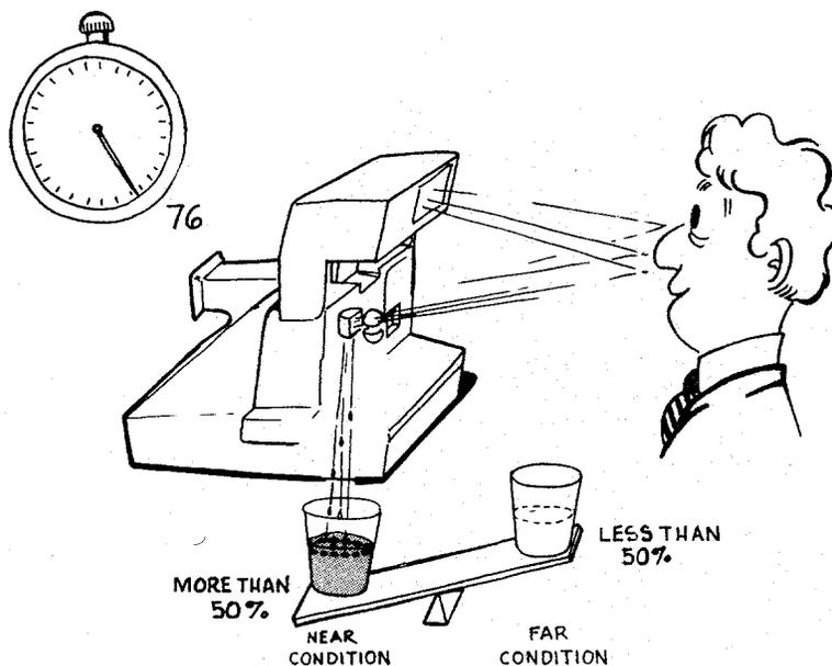
11. The camera determines whether the subject is NEAR or FAR by measuring the amount of light reflected back to the photocell 2 milliseconds after the flash has fired (76 ms into the exposure sequence). If the measurement is more than 50% of the total needed for a proper exposure, the camera decides the subject is NEAR. If the subject is NEAR, the electronics sets the clock to time-out at 124 ms.
