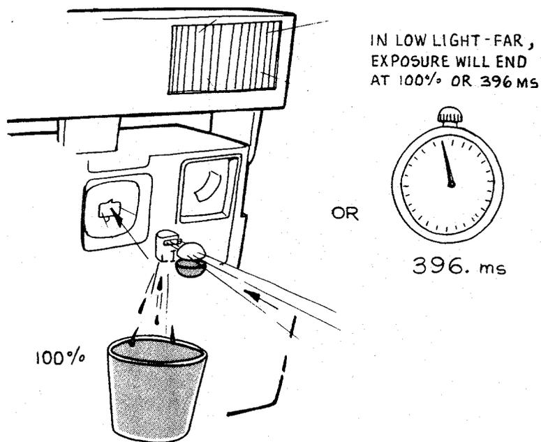
15. In a low-light FAR picture, the blades open fully and the photocell sees scene light through the photopic filter. When 100% of the necessary light is seen or when the internal clock reaches 396 ms, the flash is quenched and the shutter blades close.
