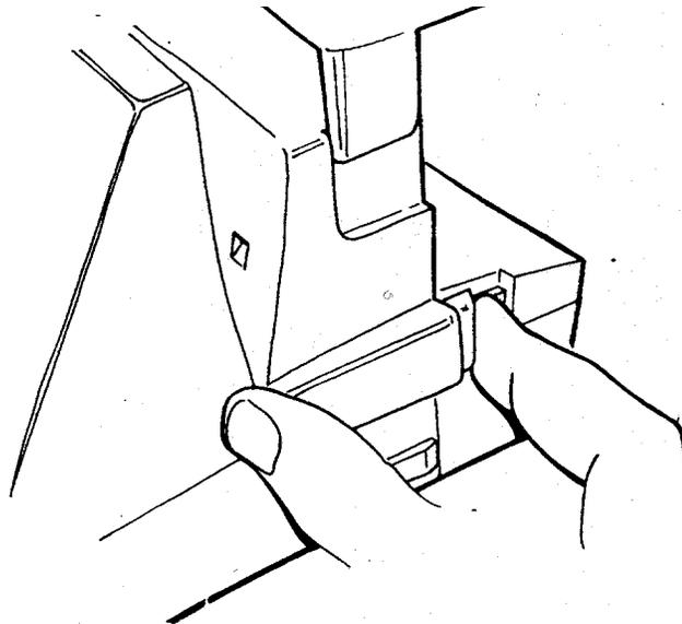
10. An alternate way to charge the flash is to lightly press the exposure button. The button can then be released. After the green LED has come on the flash will stay fully charged for approximately one minute. When the exposure is ready to be made, the exposure button is pressed in fully, in one motion.
