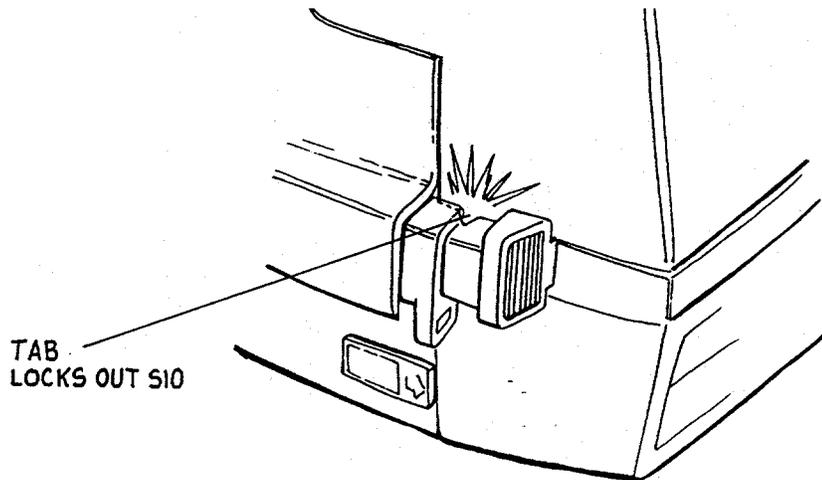
46. Finally, when the camera is in the folded position, S10 is mechanically locked open by a tab on the flash housing. This prevents the flash from being charged.
