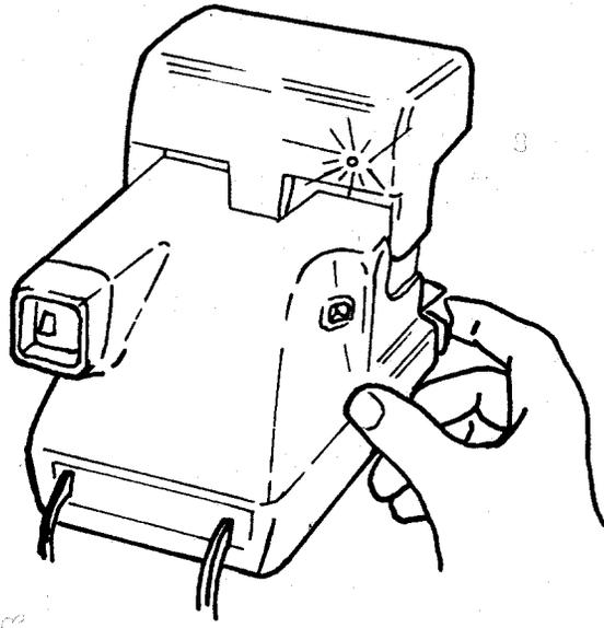
9. The flash is charged by lightly pressing the camera exposure button. The exposure mode is electronically inhibited until the flash is fully charged. When the green LED comes on, a picture can be taken by pressing the exposure button in all the way.
