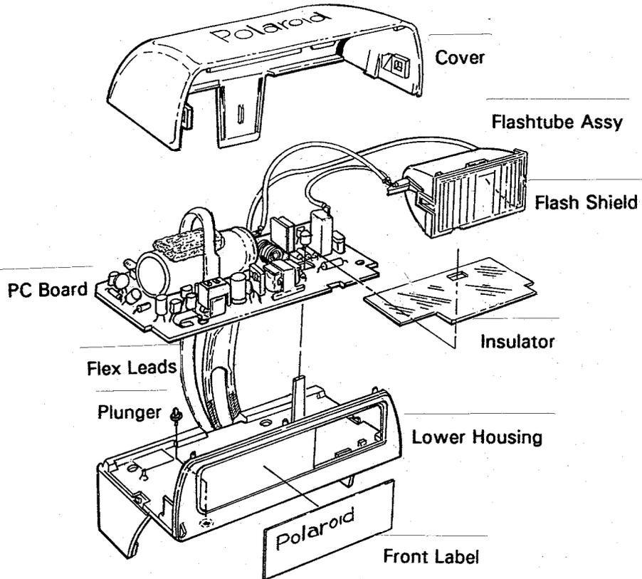
1. Remove Strobe Cover using removal tool 12633. Insert tool in hole on right side underside of Housing and tilt bottom of tool to the right (CCW) to release molded catch inside cover (A in Fig. 1). Repeat process on left side, tilting bottom of tool to the left. Lift off Cover.
