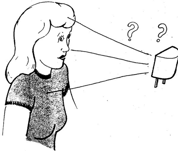
35. On the other hand, dark clothing would fool the photocell into timing out a long exposure, since relatively little light was reflected back. This would result in a washed-out face.
