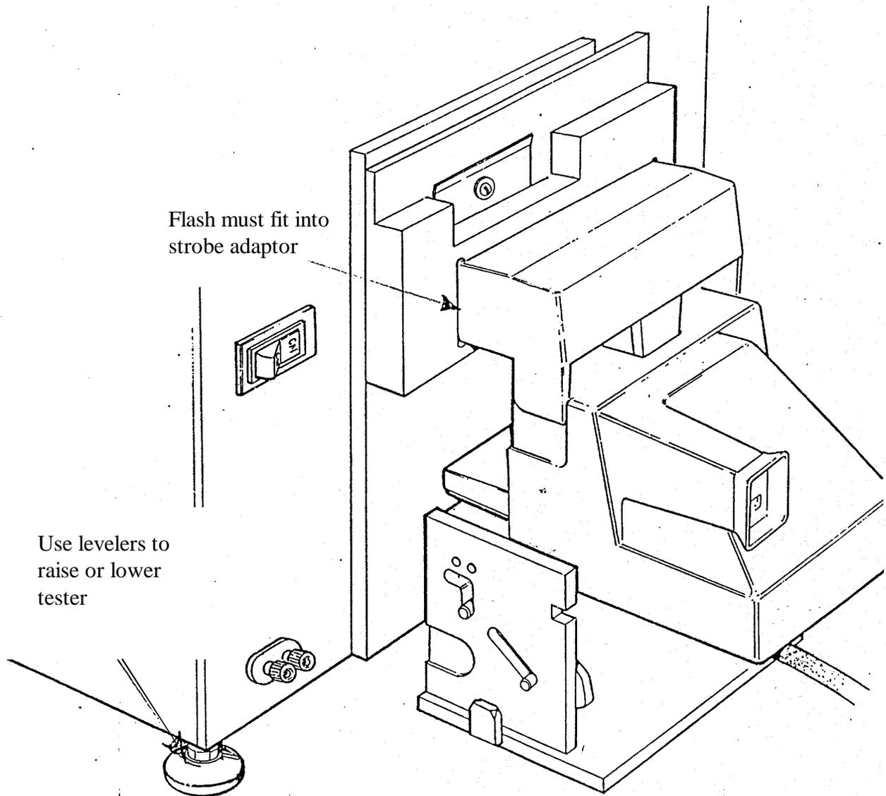
Fig. 3 Aligning Camera on Horn with Tester window
