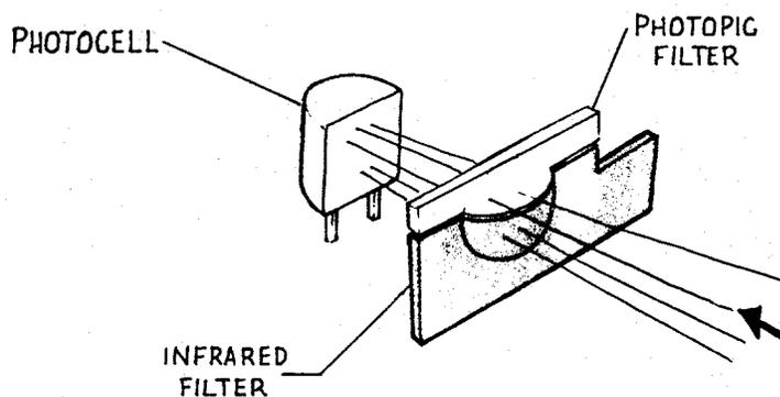
36. To overcome this problem, the Model 636 uses a photocell with a two-part filter in front of it, called a Dynamic Infrared Photometer system. The top half of the filter passes visible light which the human eye can see. This light is used to time exposures for non-flash, fill-flash, and low-light, distant scene flash pictures. The top filter is a *photopic filter*.
