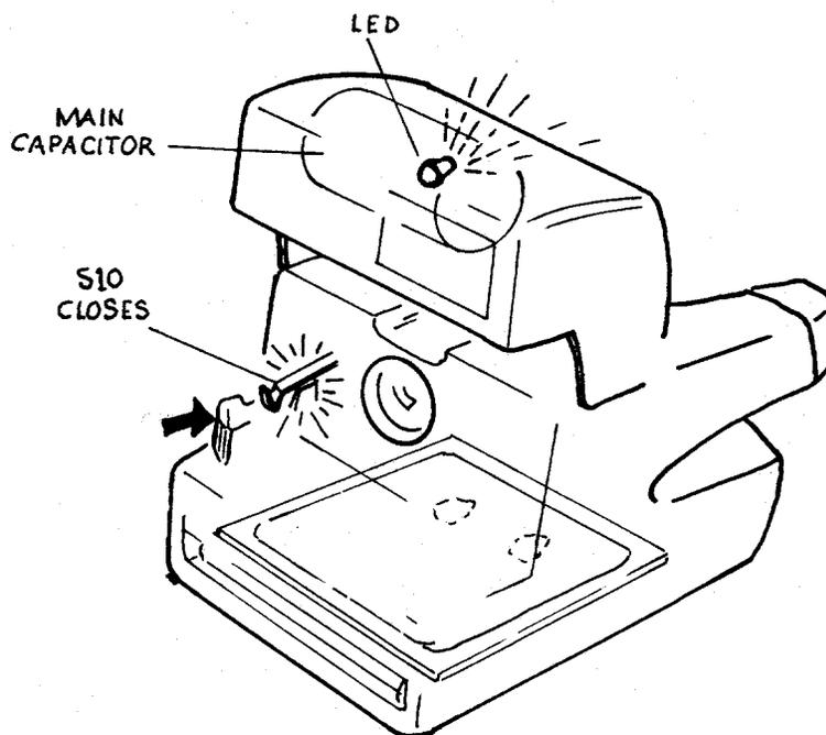
2. Lightly pressing the exposure button closes the S10 contacts, charging the strobe main capacitor.
