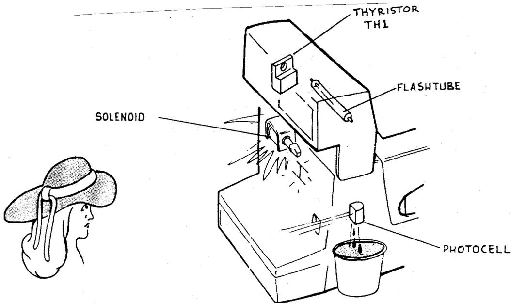
22. In the high ambient (Fill Flash) mode, the photocell makes the decision to shut down the flash and close the shutter blades. It does this when it sees the remaining 25% of the light required for a proper exposure. (This light is provided by the flash.) The camera logic signals the flash to quench and commands the solenoid to close the blades.
