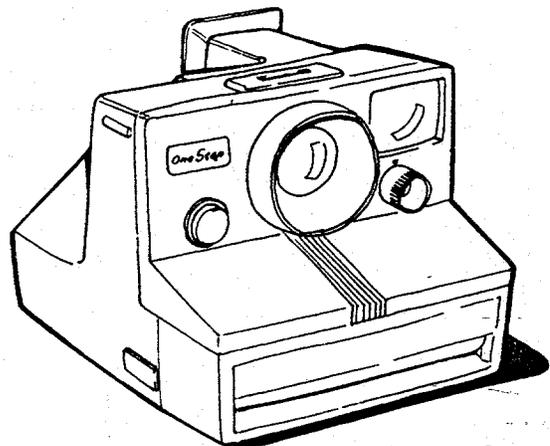
2. The Model 636 shares many of the features of the 635 and 640 Cameras. Among these are: Fixed Focus Lens, Electronic Shutter, Film Shade, Lighten/Darken Control, Empty Pack Lockout, Film Counter, Carrying Strap and a Fill Flash Capability.
