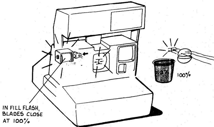
7. When the photocell sees 100% of the light needed for the exposure, the camera electronics orders the flash to quench and the solenoid to energize. The solenoid then pulls the blades closed.
