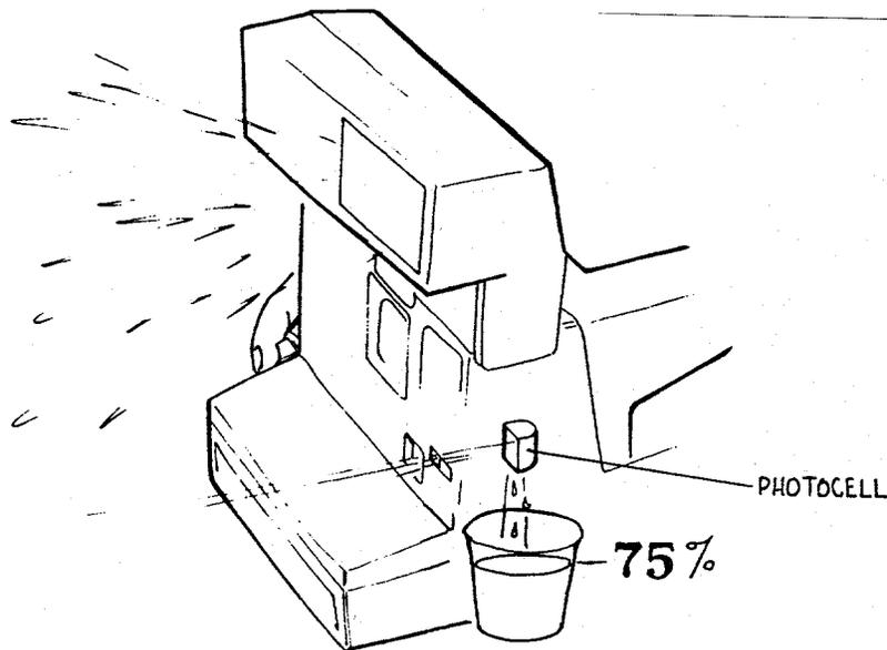
20. In the high ambient or Fill Flash mode, the photocell measures scene light. When it sees 75% of the total light required for a proper exposure, the photocell fires the flash.
