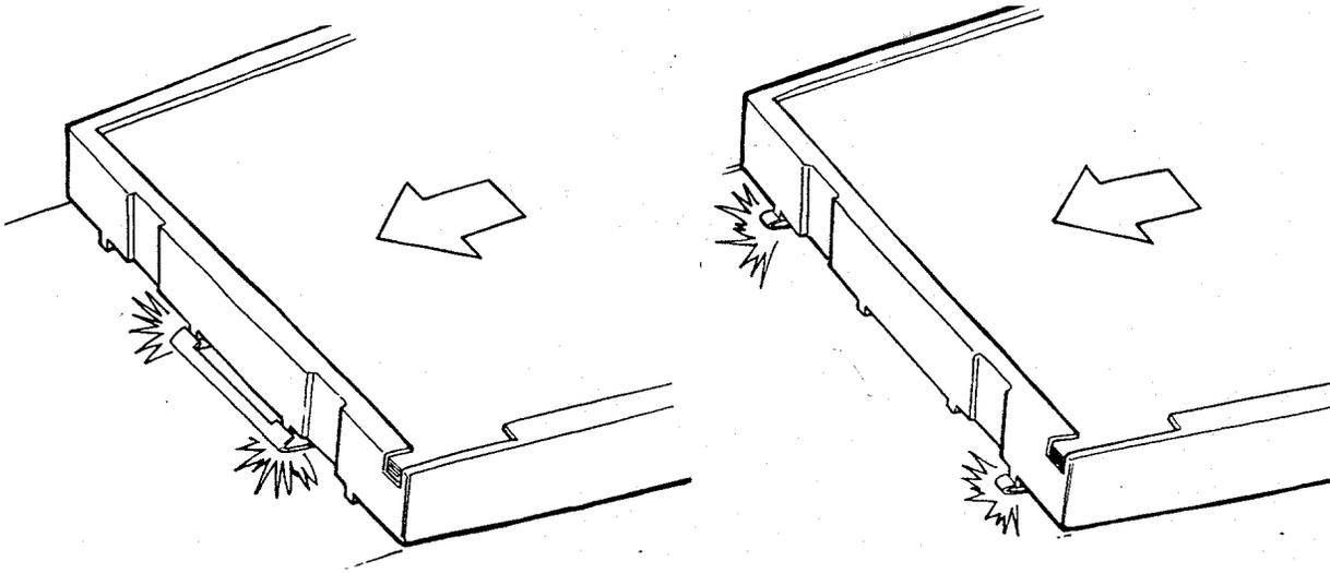
5. On the other hand, a 600 film pack cannot be inserted into an SX-70 style camera since the tabs on the pack are held back by the older style pack springs.
