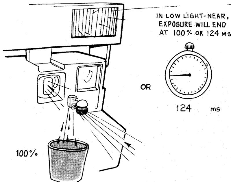
12. In a low-light NEAR picture, the blades open partially so that the photocell is measuring infrared light through the infrared filter. The flash is quenched and the shutter blades closed either when the photocell sees 100% of the light needed for a proper exposure or when the internal clock reaches 124 ms.
