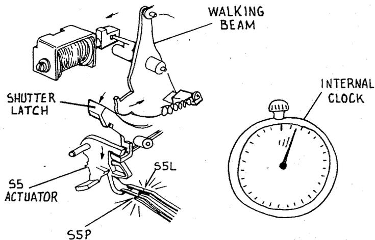
4. As the solenoid pulls in, it releases the walking beam from the shutter latch. The spring-loaded S5 actuator drops down, closing the S5P and S5L contacts. S5L starts an internal clock. The camera electronics signal the solenoid to deenergize.
