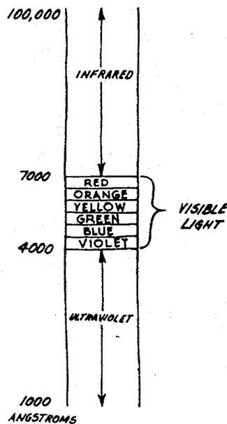
38. This chart shows the light spectrum. In the infrared region of the spectrum, a strange phenomenon occurs. The light reflected off just about all materials is equal. Therefore, the light passing through the infrared filter is balanced, preventing the photocell from being fooled by contrasting levels of light or dark subject matter.
